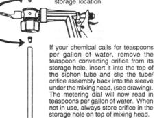
base of mixing head, and thread bottle into head. Attach a water hose to handle and turn on water. When you squeeze the handle you will automatically be spraying the proper number of teaspoons or tablespoons per gallon of water.
